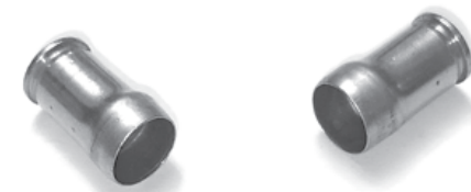
.32 ACP cartridges fired from a .380 ACP chamber.
