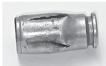
A 10mm fired in a .45 ACP chamber.
