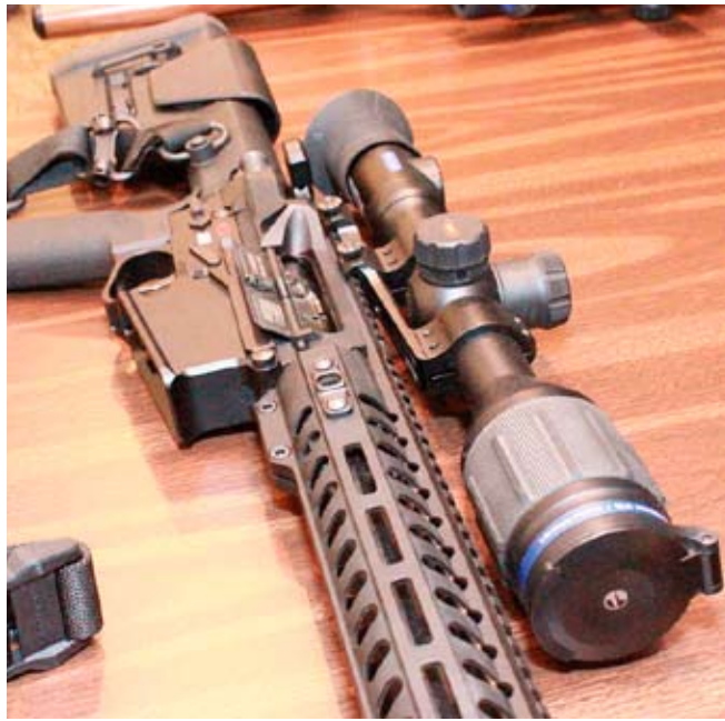
This is what $5000 worth of thermal imaging scope looks like. It's not a lot bigger than a conventional scope only it allows for accurate engagement in both day and night.
