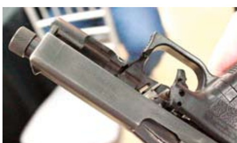
A blown-up Glock from Charleston. A double-powder charged reloaded cartridge was to blame. Avoid unknown reloads.
