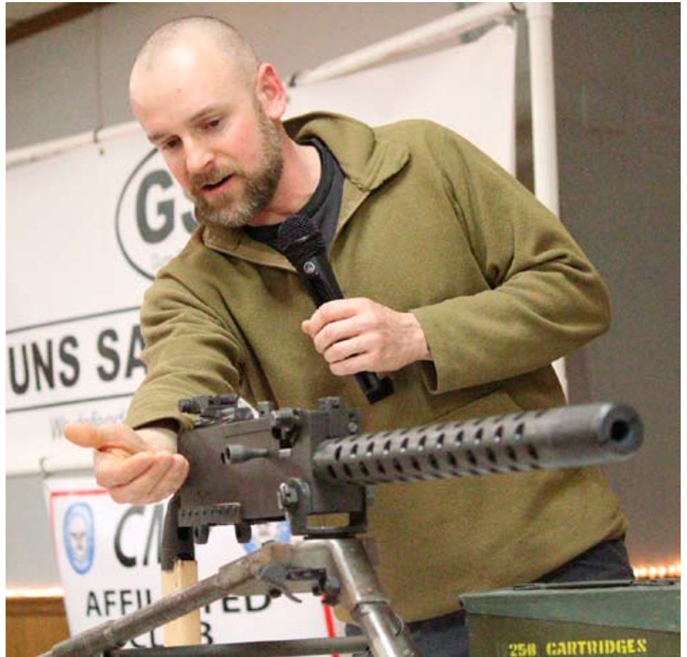
Eli Slaminko with one of Central Illinois' biggest 'ghost guns' - a Browning 1919 converted to semi-auto. It stands as one of the rarer .30-06 versions. The Israelis ended up with a lot of 1919s and eventually converted them to 7.62 NATO before sending them to America. This one, however, is an original .30-06.
